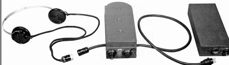
General view of the Crosley developed prototype SCR-295 receiver which had a separate battery box.
