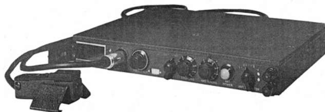
General view of the transmitter with a miniature Morse key which was stored in the compartment at the left side of the front panel when not required (above).
